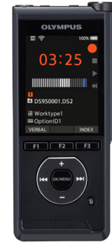
Figure 12: The DS-9500 Digital Recorder, offered by Olympus, features Wi-Fi technology that allows users to quickly send dictations without needing to physically plug into a computer and a noise canceling system to improve dictation management efficiency. (Image provided by Olympus)
