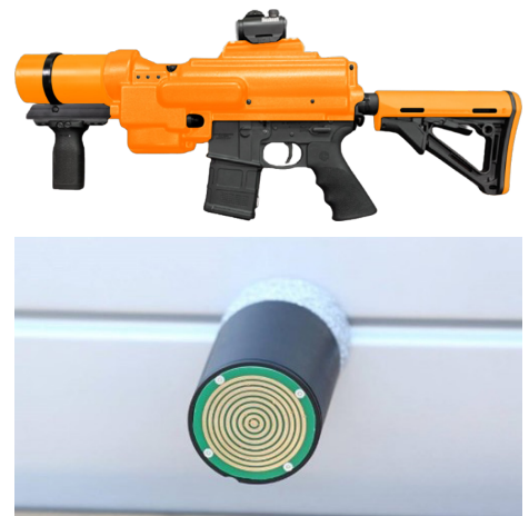
The Guardian, a handheld GPS launcher, is one of two GPS tracking devices offered by StarChase and is employed to follow a suspect’s vehicle to a controlled environment for de-escalated apprehension (photo provided by StarChase).
