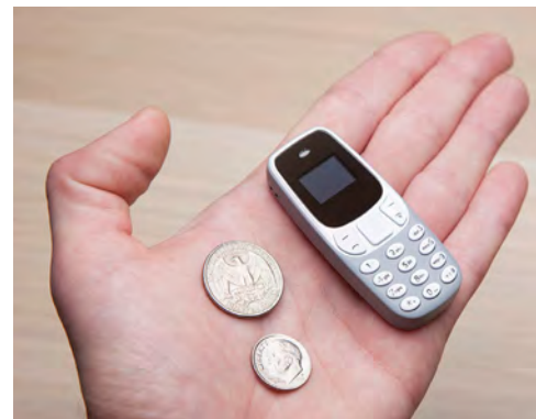
Figure 2: A mini cell phone approximately 5 cm in length is easily hidden, can transmit phone calls, and is Bluetooth capable.
