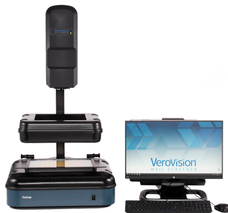
Figure 4: VeroVision Mail Screener, offered by ChemImage, uses imaging spectrometers and sensor technology to detect drug contraband found in mail.
