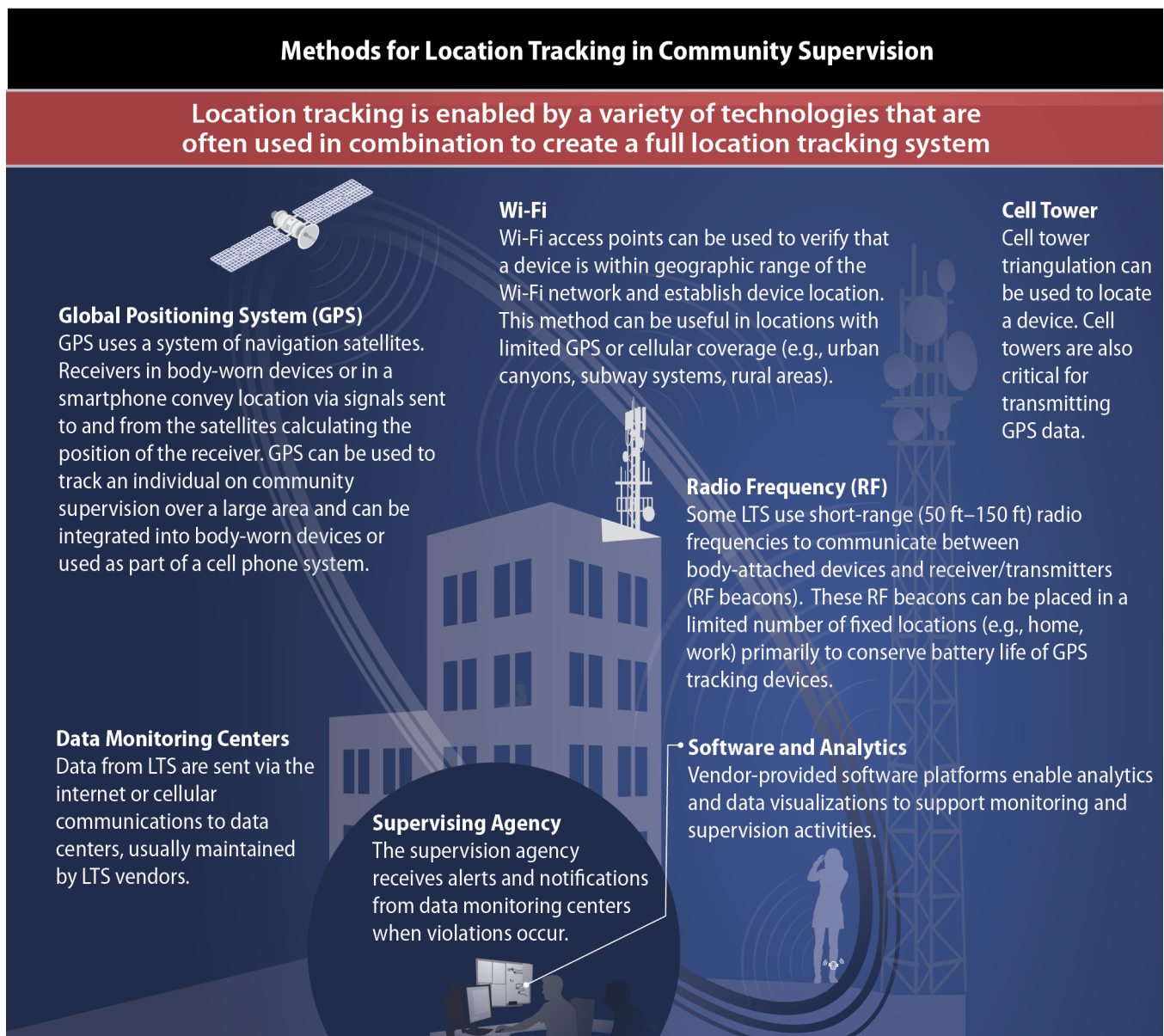
Figure 4: LTS use various technologies to determine the location of a monitored individual and transmit that information to supervision officers.
