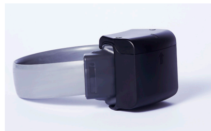
Example: Several products like GEOSATIS’ Electronic Ankle Bracelet, Securus Technologies’ BLUtag, and Buddi’s Smart Tag (above) come with charging “collars” that attach to the device and wirelessly transfer power.
