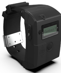
Example: S911 Enforcer from Laipac provides alerts to the monitoring center when an individual enters or exits a predefined area.
