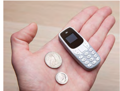
Figure 2: A mini cell phone approximately 5 cm in length is easily hidden, can transmit phone calls, and is Bluetooth capable.
